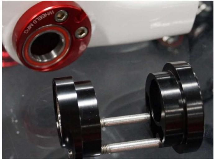
If that doesn't work, I'd install one of these Wheels Manufacturing bottom brackets instead. Since it threads together on itself, it keeps everything in alignment.
